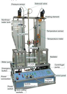
The system includes demo software for basic commissioning, PI level control, PID temperature control, and non-linear control. These features accelerate the learning curve for developing process control PLC programs in a realistic training environment. The BPCLS is an ideal solution for individuals and organizations that want to improve their process control skills and gain a deeper understanding of industrial equipment and processes.
