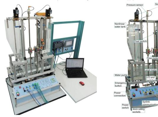
The system includes demo software for basic commissioning, PI level control, PID temperature control, and non-linear control. These features accelerate the learning curve for developing process control PLC programs in a realistic training environment. The BPCLS is an ideal solution for individuals and organizations that want to improve their process control skills and gain a deeper understanding of industrial equipment and processes.
